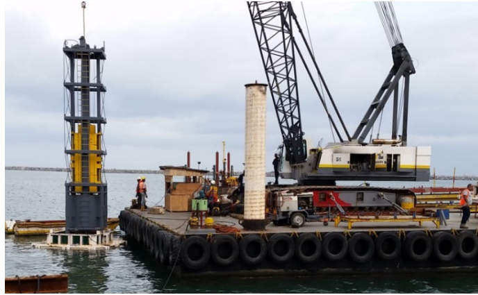
Figure 3. Photographs of the mounted drop weight device for offshore dynamic load tests (GeoDynamica, Inc. 2015b).
