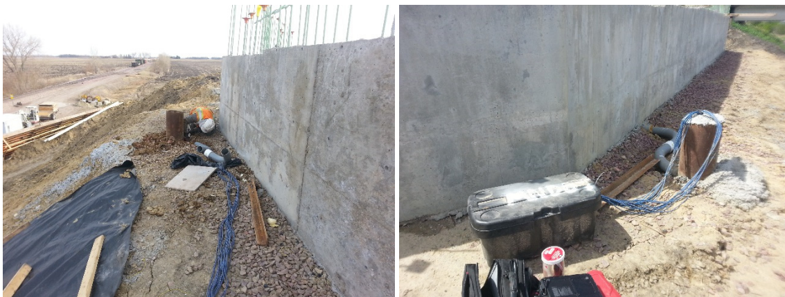
Figure 8. One of the two sacrificial reaction piles (SRP-2) from a load test at this site can be seen in front of the west integral-abutment pile cap. A set of gages in the same arrangement as in the test pile was installed to repurpose this pile for dragload characterization at the site.
